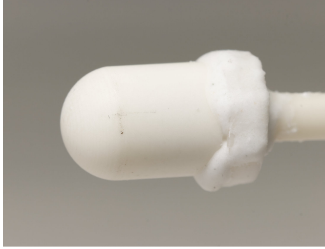
Figure 2.5: Ceramic cap of a Bdot probe which is inserted into the LAPD to measure magnetic fluctuations
